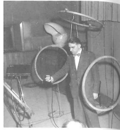
Pierre Henry, pupitre d'espace , a device utilizing induction coils, built by Jacques Poullin in 1951 at Pierre Schaeffer’s suggestion
